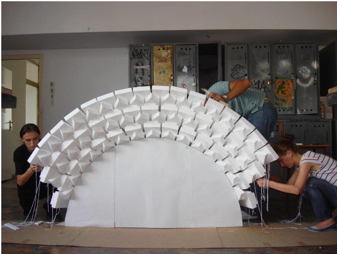
Fig. 3: Scale 1/1 model of an arcade for the reconstruction of the drum and dome on the church in Berislavesti, front view
