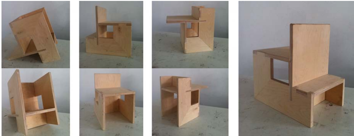
Fig.10 – The multifunctional furniture item above used a thicker panel, while finger joints were reduced to maximum. They were reducing the complexity of execution process and they conferred enough rigid and resistant structure for object's usage. This furniture can be used as storage (i.e. for reviews and magazines), as chair or as a small coffee table – all the functions depends on the position it is placed.
