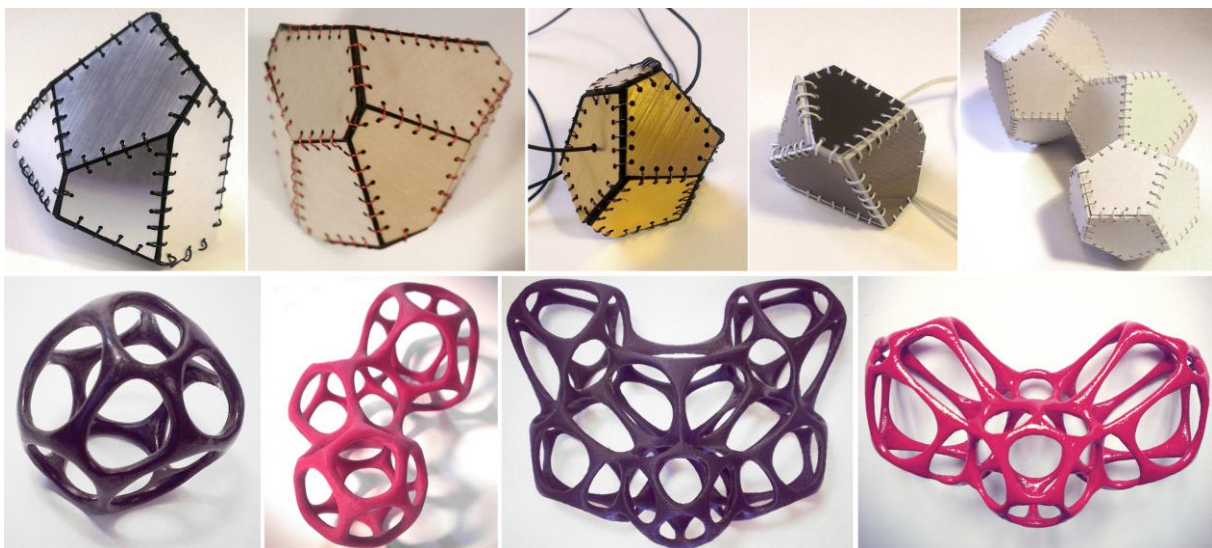
Fig. 4. The objects that explored two different fabrication methods. The first series are laser cut and articulated by sewing the faces together. The second series are 3D printed. Both are interpretations of the same cellular aggregation principle.
