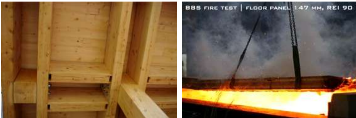
Images I-09 and I-10. Example of using fireproof wood panels (Left) and test examples on BBS boards type for fire resistance (Right). Source of images: the author's personal archive.
