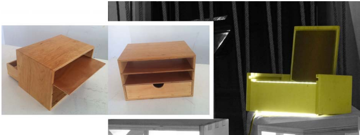
Fig.7 – Objects using the dado joints – they confer them a sliding system without any other added accessories. The box has sliding shelves to place A4 paper on them (left) and the mirror top of the jewellery box can slide off the box when it is moved to close it (right).
