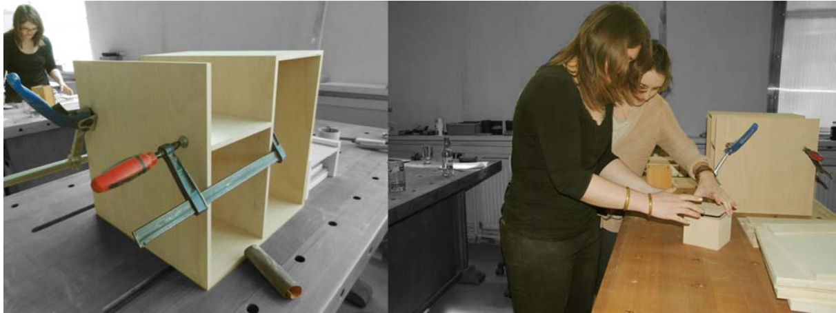
Fig.3 – Each type of joint or assemble operation impose steps to be followed. Adapted tools for gluing stages can be seen in the snapshots above. Assembling steps have to be established and followed accordingly; if steps are not respected there can be situations leading to failed results.
