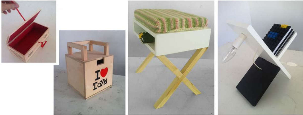
Fig.6 – [1] and [2] were simple boxes that were getting some graphic interventions such as poker work or painting. [3] This furniture piece introduced lacquering and added an upholstery element that can increase its functions from a simple storage console to a potential sitting place. There were used halved joins for legs and simple joints for carcass. [4] By using hidden simple joints applied on MDF panels instead of wood, this object was totally lacquered. It was also the first object adding the lighting function to a storage small furniture item.
