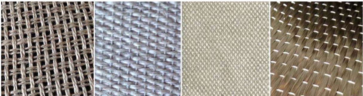
Fig. 3_FIDFLAX GRID 300 HS20@: balanced grid flax fiber sheet for structural strengthening; FIDFLAX UNIDIR 430 HS43@: unidirectional high strength flax fiber sheet for structural strengthening; FIDHEMP UNIDIR 240 HS22@: unidirectional high strength hemp fiber sheet for structural application; FIDBASALT UNIDIR 400 C95@: unidirectional basalt fiber sheet for structural strengthening. Image courtesy FidiaTechnical Global Services.
