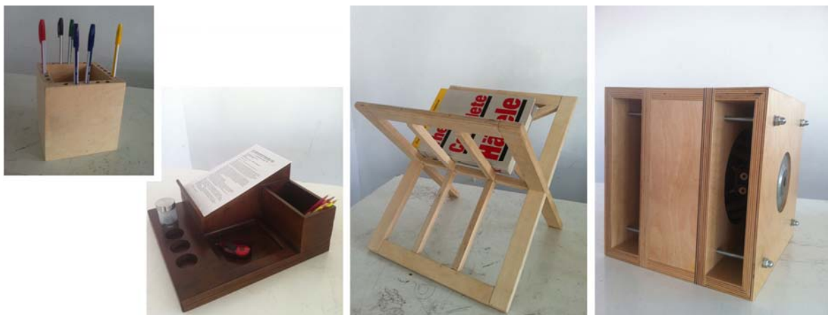
Fig.5 – [1] and [2] multifunctional objects to be placed on a desk, being used for paper, pens, paperclips and other office accessories, were executed with simple cuts, drills, 45° angle joint (mitre joint) and glue. [3] Dowel and bridle joints were leading to a framed object that could keep different objects in different positions stocked. [4] Simple joints but complex concept – a functional wooden loudspeakers carcass.
