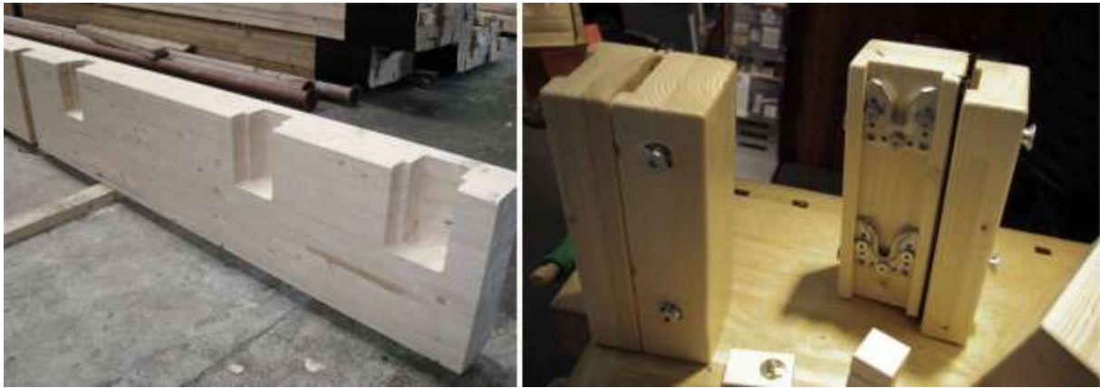
Images I-07 and I-08: Laminated beams with holes for positioning side elements cut with numerical control machine based directly on CAD files (Left). Metal connectors providing rotational stability of the wood (Right).
