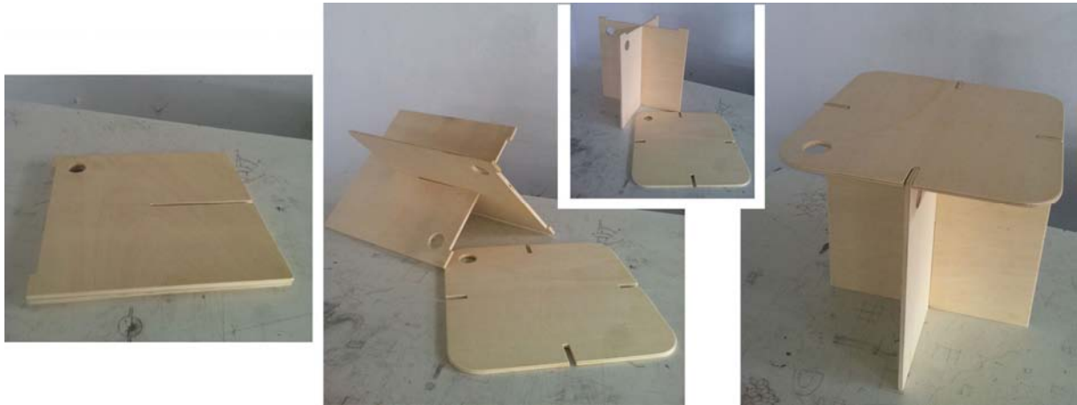
Fig.8 – The helved joints of three similar wooden panels could lead to the concept of a folding chair. The joints permit assembling and resembling the chair, conferring the needed structural strength at the same time.
