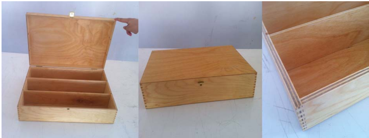
Fig.9 – A storage box for wine bottles was executed using finger joints. Their number and sizes implied much more work, but they also confer better resistance of the frame, giving the opportunity to use a very thin panel. The dado joints inside permit the raster to be modified with easy, depending on bottle's size or box's usage.
